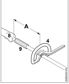
Fit the loop handle (4) at a distance of (A) approx. 20 cm (8 in) forward of the control handle (8)
